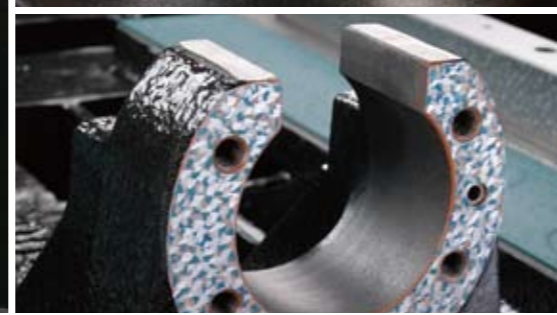
Hand scraped contact areas, minimal axis protection with maximum stroke.
