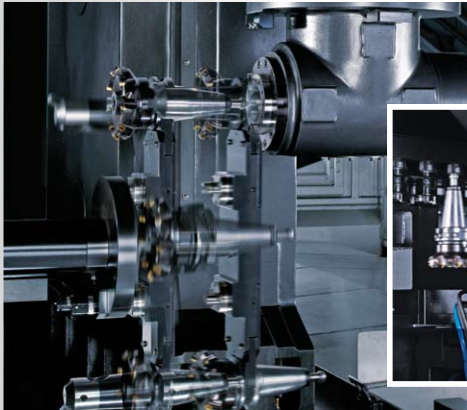
Automatic tool exchange in horizontal ( C to C 50 sec.); In vertical (C to C 35 sec.)
